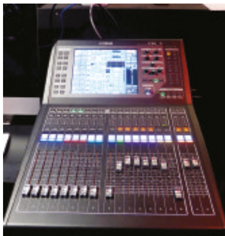
Mixing is via a Yamaha QL1 16-channel console with an MY8 A096 analogue expansion card
