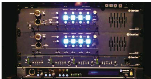
The Clear-Com FreeSpeak II Base II station can support up to 25 belt-packs via ten transceiver antennas and two splitters
