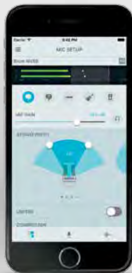
MV88 Settings Screen Select DSP Preset, Mic Gain, and Adjustable Stereo Width
